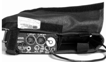
side view showing battery pouch below mixer
