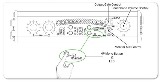
① Optionally—via a DIP switch setting—the stereo signal from the computer may also be summed when Headphone Mono mode is engaged.
