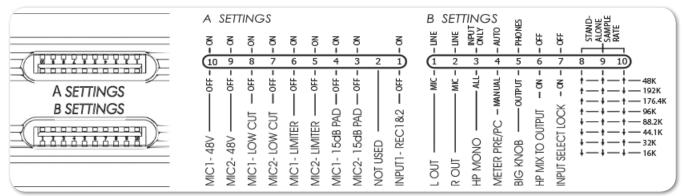
In the following descriptions, "up" refers to the direction opposite the numerical labels on the switch casings.
