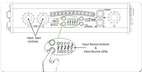
① The Input Source buttons may be locked—via a DIP switch setting—to prevent accidental switching of the input sources.
