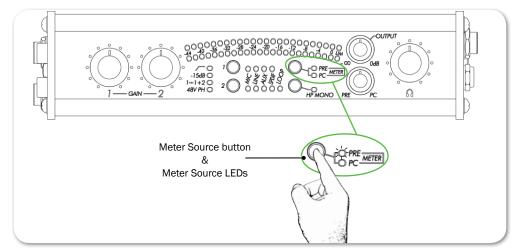
When the meter source is set to PC the meter displays the audio level for signal
